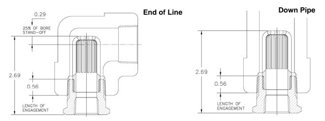
1.0" - Pipe Fittings Shown, all other variants are free install and have no restrictions with the In-Flow segregator positioned well below the concentric flow point. This has been enabled due to the high level of flow and protection given by the In-Flow Segregator which can protect a 3mm exit orifice to 17.8mm without affecting the K-Factor exit of the sprinkler head, an industry first.
