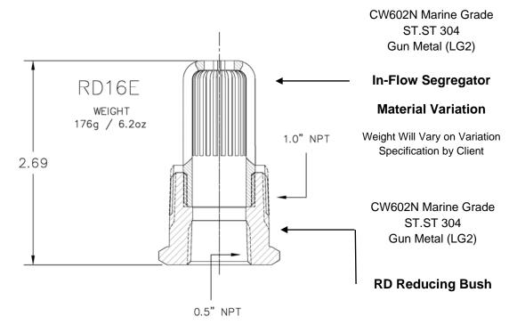
The RD16E Variation is to be used on all pie sizes and locations above a 1" Tee, the RD16T is required to be utilised to mitigate the risk of pipe line blockage. The RD16E is to be installed as below for a 1" Pipe with the (make-up) to be mimicked for all other pipe variations as shown in both the ELBOW and DOWN PIPE below.
