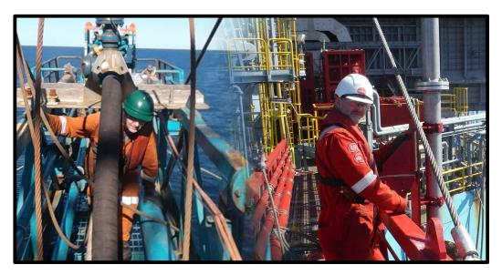
Personnel should never have to work under the conditions shown on the Left when there is an engineered solution available. This Expro Operator above and the Schlumberger Operator below are visibly struggling to make it along a walk way designed so allow for safe ingress and egress.
