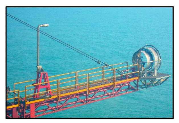
With a full 360° Rotation Vertical and Horizontal the system can be stowed very easily between well test operations to avoid crane operations.
